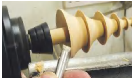
▲ Pic.8 To improve the finish on the underside of the branches, make a very light cut with the skew on its side, to create a shear cutting effect
